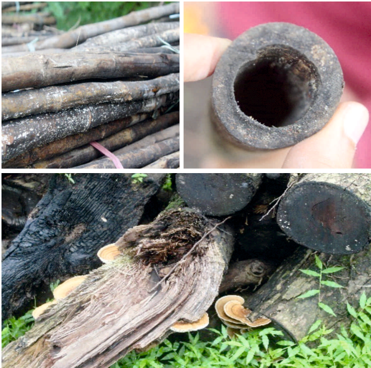
Figure 2. Reduction on market value of wood due to fungal infestations, degradation, and staining
