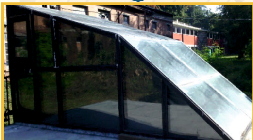
Head based storage Solar Kiln
